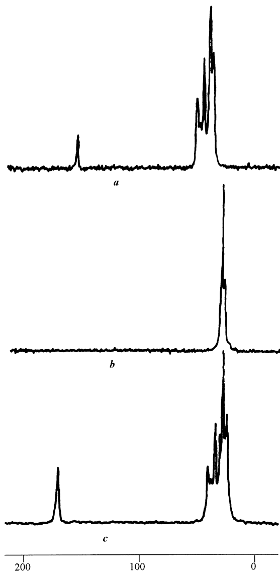
Fig. 10. ^{13}\text{C} CP-DD-MAS RMN spectra of (a) PA-6; (b) EVA8; and (c) PA-6/EVA8/APP.
